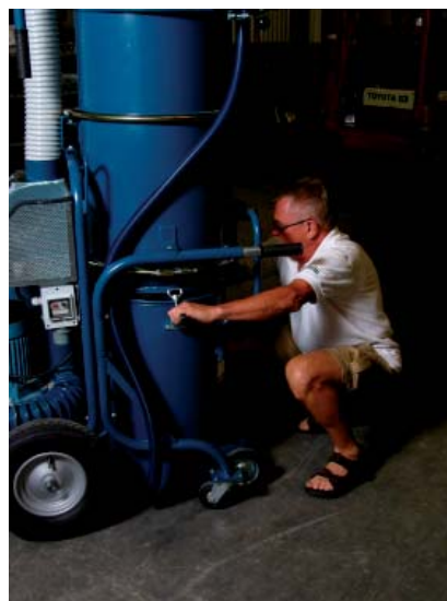
The container is attached to the machine by two fasteners.
